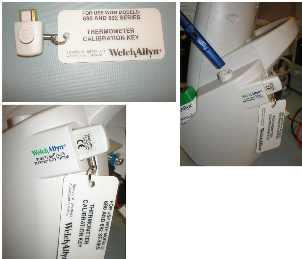
3. Insert and then remove probe from probe storage channel to reset thermometer.
