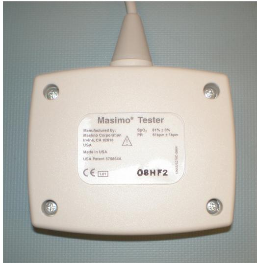
1. With the UUT OFF, orient the Masimo Tester such that the mini-D connector mates with the SpO2 connector on the UUT; or use appropriate Masimo extension cable to connect the Masimo Tester and UUT.
