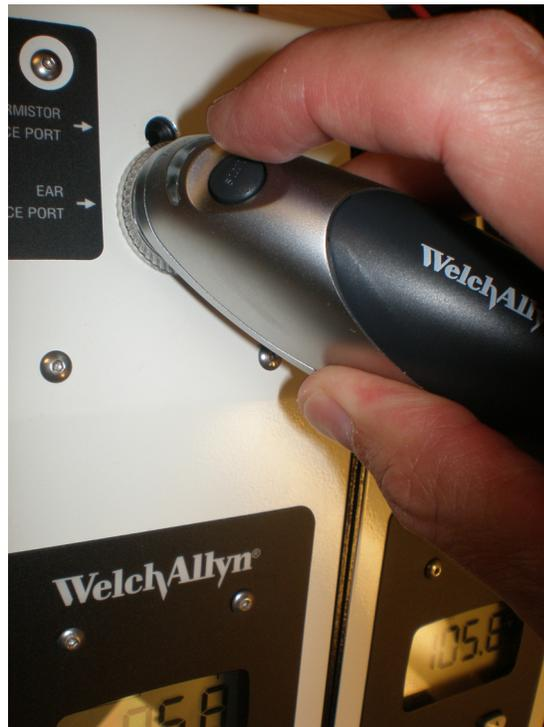
4. Leave the thermometer in the 9600 Plus Calibration Tester until you hear a beep. Remove the Pro 4000 Thermometer from the 9600 Plus Calibration Tester and read the temperature in the thermometer's display.
