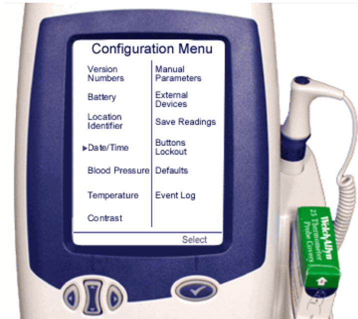
4. Scroll to **Date** on the UUT and select. Using the navigation keys, adjust the correct date and select. Scroll to **Time** and select. Using navigation keys, adjust the correct time and select.
