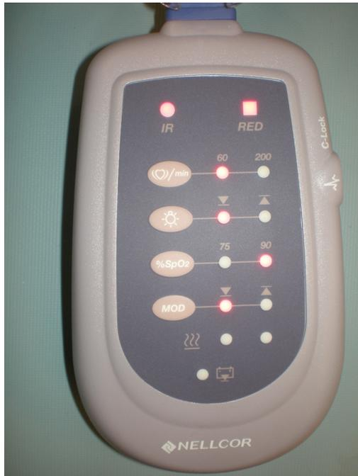
1. With the UUT ON and completely booted, orient the simulator such that the connector mates with the SpO2 connector on the UUT; or use appropriate Nellcor extension cable to connect the simulator and UUT.
