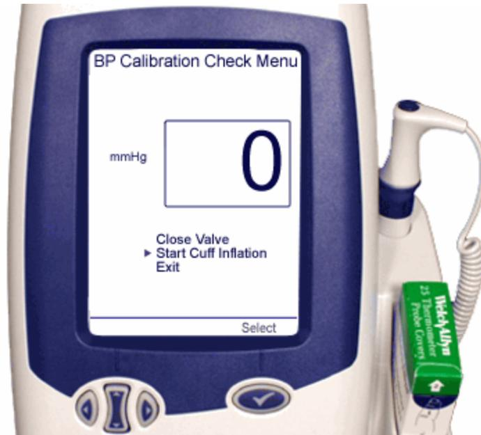
8. Inflate the pressure up to 250 mmHg. Select the **Stop Pump** on the UUT to stop the inflation. Fine tune the pressure reading to 250 mmHg with the squeeze bulb.
