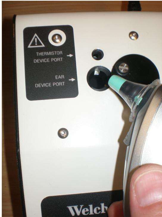
3. Wait approximately three seconds, press the thermometer **start** button, and watch for the “Exac Temp” light to flash.
