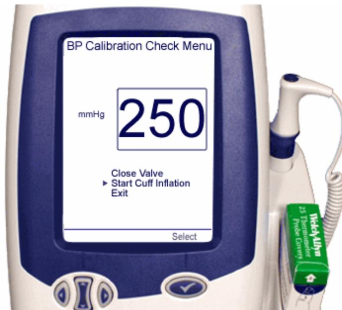
9. Check the reading on the pressure meter against reading on the UUT.
