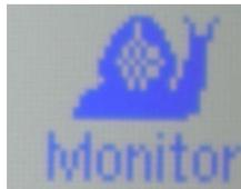
5. After the UUT enters "Monitor" mode wait for approximately one minute or until the temperature on the thermometer is stable for ten seconds.
