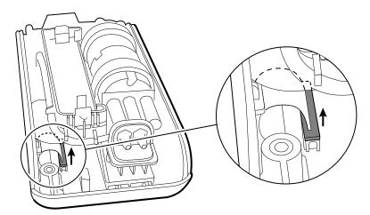
Remove the flex cable from the ZIF connector.
