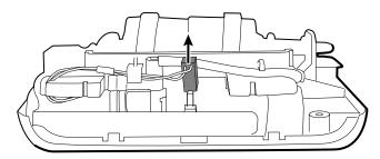
2. Disconnect the step valve manifold from the step valve on the blood pressure board.
