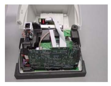
**NOTE:** Observe how hose fits in E-Pac Foam. The hose fits over wiring keeping wiring secure.
