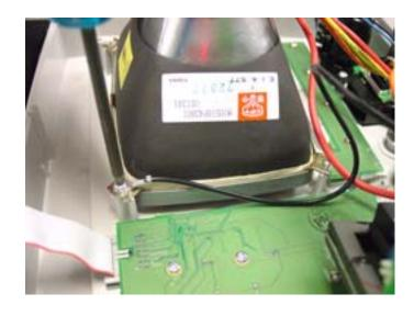
**NOTE:** The CRT and deflection PCB are factory tuned as a unit and are sold only together as a unit.
