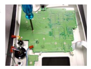
**NOTE:** Notice the correct orientation of CRT screw and washer.
