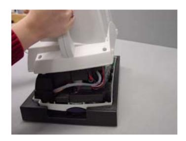
3.3 Flip the housing forward. Take special care not to damage any cables.
