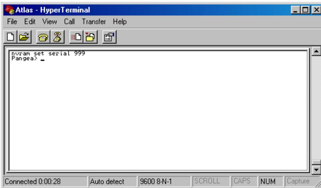
Figure 2-16. Pangea screen after you have downloaded the nvrAm set serial command.
