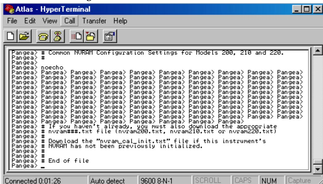
Figure 2-12. Pangea screen after opening the *nvram\_common.txt* file.
