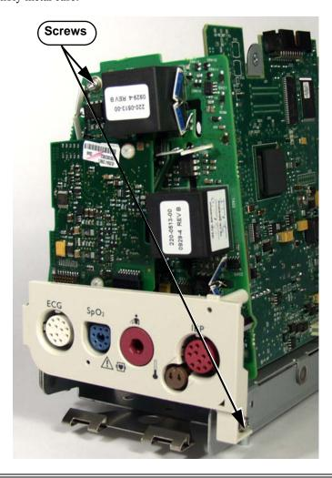
5 Pull the front end assembly away from the 40-pin connector on the side of the main board.
