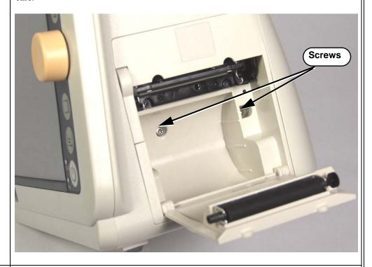
Place your thumbs on either side of the recorder case and pull it straight out of the assembly and away from the recorder connector on the main board.
