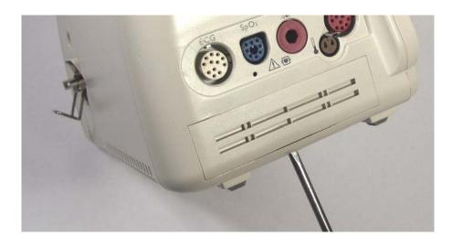
Holding one hand over the battery cover, while you twist the screwdriver slightly to release the battery cover from the case.
