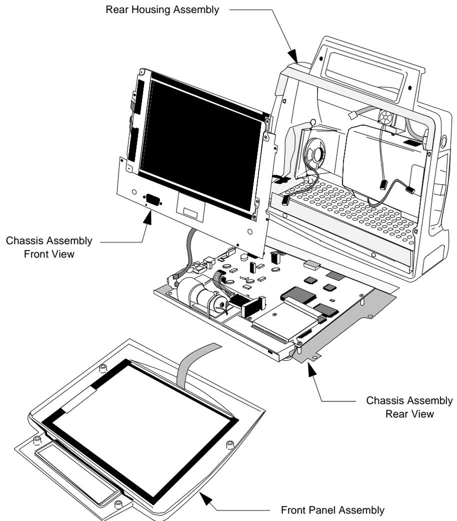
Figure 5-3 Exploded View of the TeleMon Monitor
