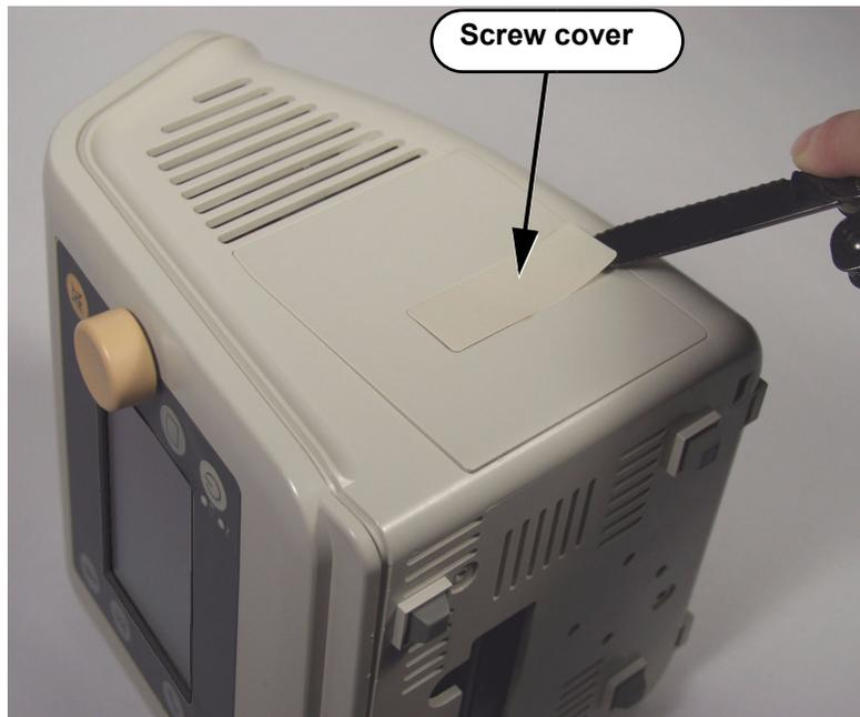
2. Remove the two screws and pull the faceplate straight away from the monitor.
