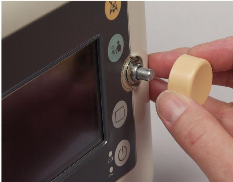
3. Remove the locking nut and washer.
