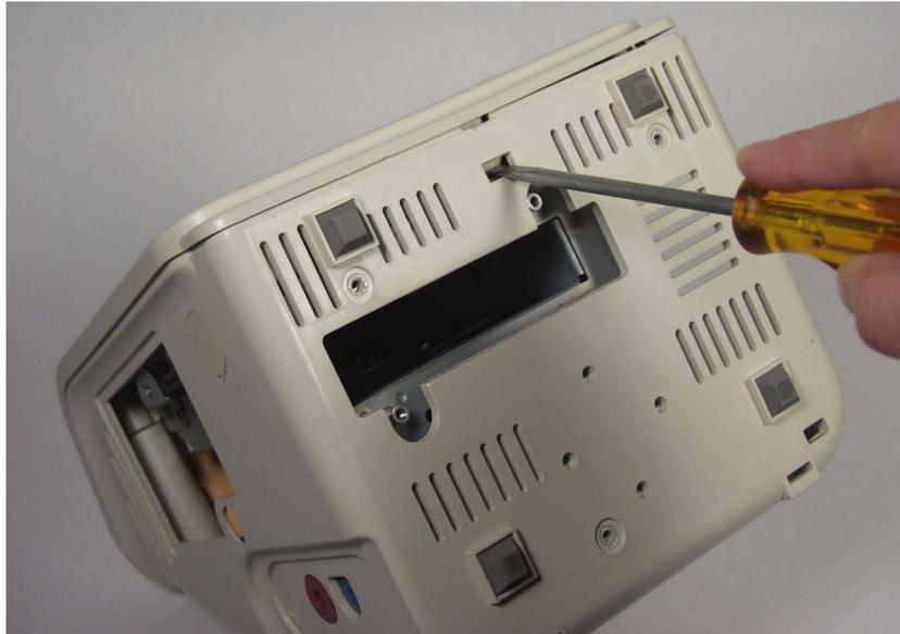
9. Lift the front panel assembly carefully and slowly over the handle and pull it away.
