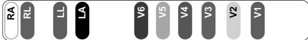
Figure 6-16 12-Lead PIM IEC Lead Wire Labeling
