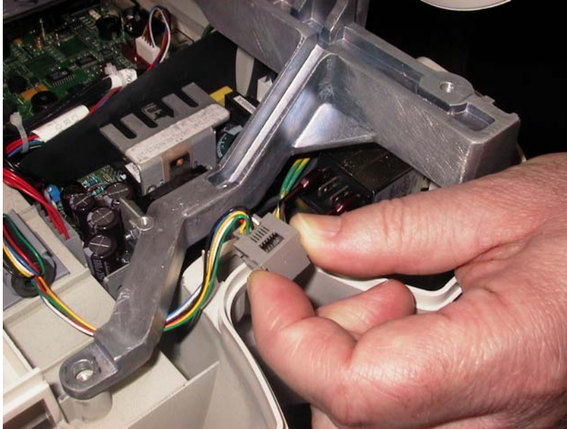
Figure 6-82 Removing the PIM Connector
