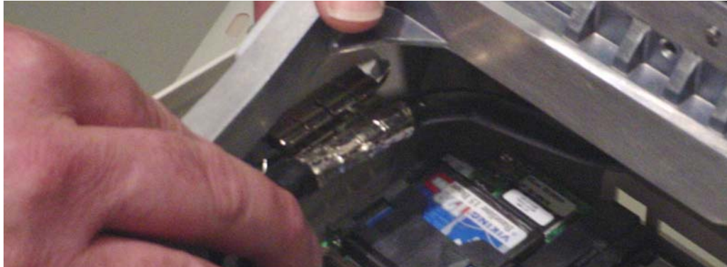
Figure 6-43 Inserting the Display Cable Into the Bracket
