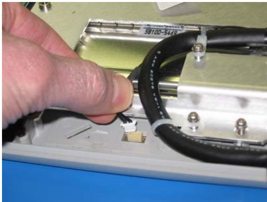
Figure 6-47 Disconnecting the On/Standby connector
