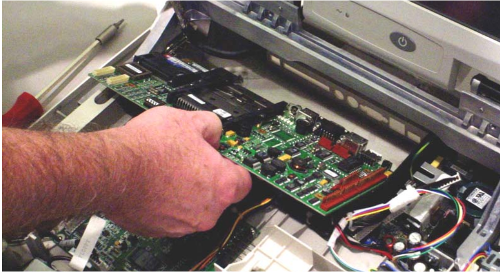
Figure 6-72 Lifting Out the Main Control Board
