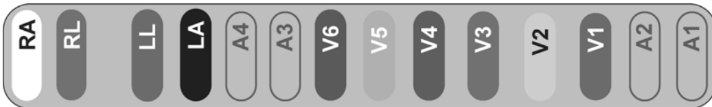
Figure 6-18 16-Lead IEC PIM IEC Lead Wire Labeling
