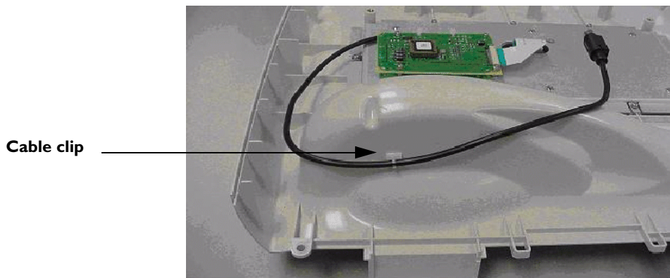
Figure 6-36 Keyboard Cable Routing
