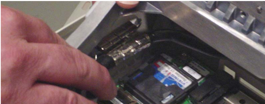
Figure 6-39 Removing Display Cable From Bracket
