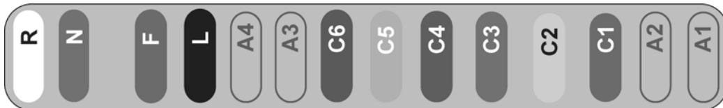
Figure 6-18 16-Lead IEC PIM IEC Lead Wire Labeling
