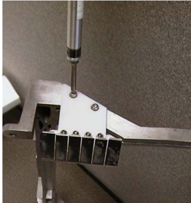
Figure 6-93 Removing the Display Cable Bracket From the Hinge Bracket
