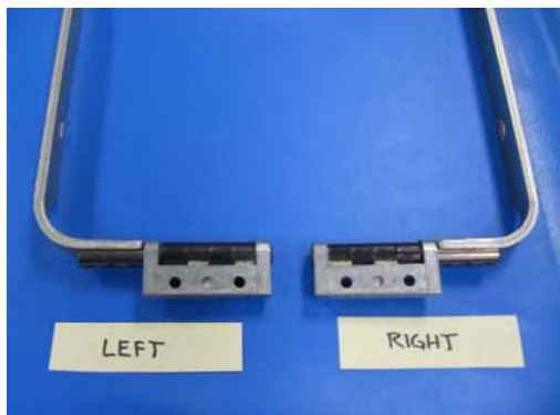
Figure 6-51 Right and left hinge assemblies
