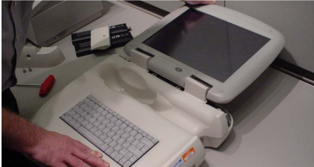
Figure 6-33 Rotating the Display Down
