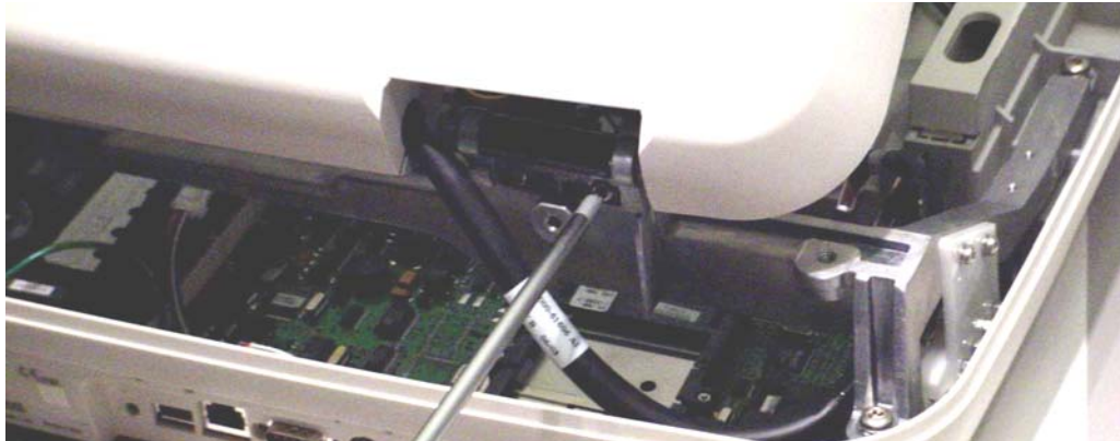
Figure 6-41 Removing the Hinge Screws
