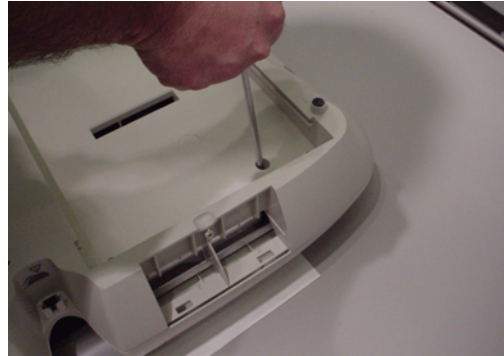
Turning cardiograph upside down and removing screws
