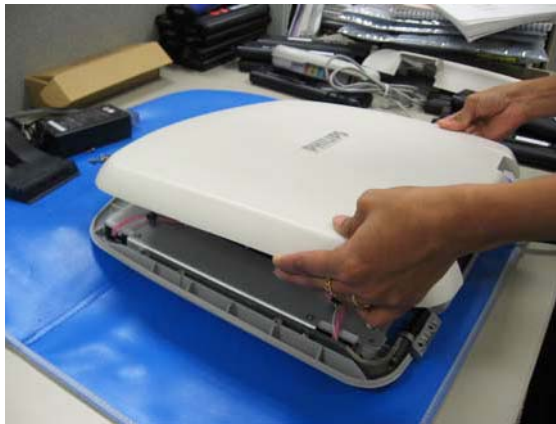
Figure 6-46 Lifting the rear cover off of the display
