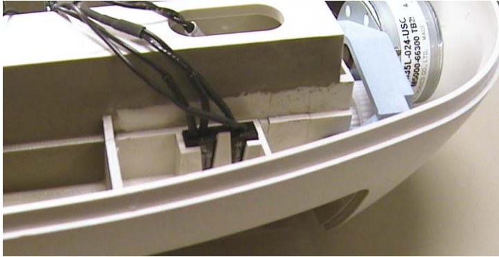
Figure 6-90 Top of Form Sensor
