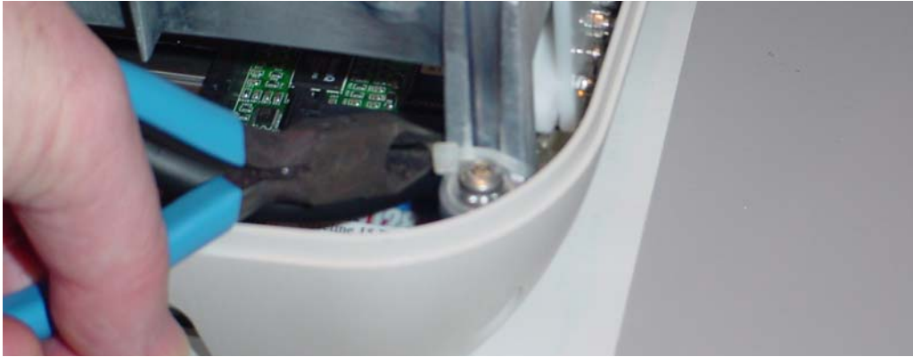
Figure 6-38 Cutting the Tie Wrap
