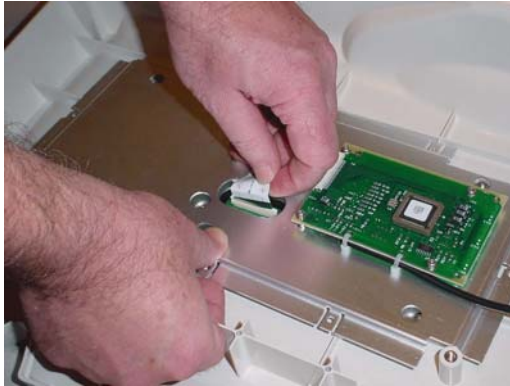
Figure 6-53 Disconnecting the Flex Cable
