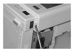
**Step 8** Stand the Monitor up again and gently lift the Monitor Bezel up and out. Gently let it rest in front of the Monitor. Be careful. It still has a cable attached:
