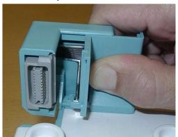
4 Turn the MSE around and insert part C into the bottom part of the link bar. When you hear a click, part C is correctly inserted.
