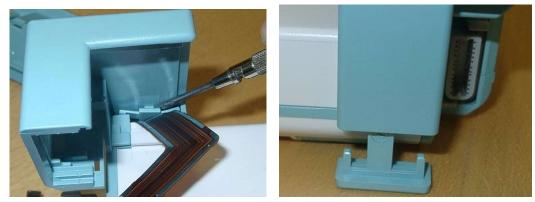
7 Lift part A upwards. It is fixed in a dovetail. Be careful with the MSL flex.
