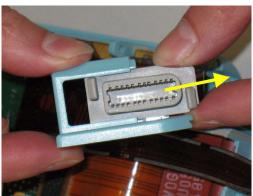
**3** Remove the flex cable connector on the MSE board. Be careful not to bend any pins on the female part of the MSE connector.
