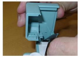
2 Make sure the MSL Flex connector is positioned in the correct slot (See indicated slots below). Then push it gently into part A.
