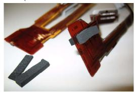
5 Insert the flex cable connector into the female receptacle on the MSE board. Check from the side and the front that the connector is inserted correctly (there is no mechanical guidance) and that no pins are bent, otherwise you may damage the MSE when powering it on.
