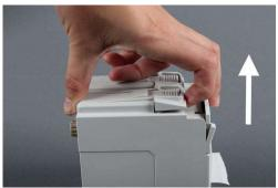
3 While lifting up, push the snap lock once with your thumb in the direction of the door in order to release it from its rail. Then slide it all the way out.
