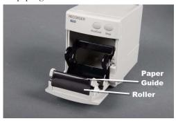
2 Carefully remove the paper guide from its position by pulling the gray holder to the left and the paper guide to the right.
