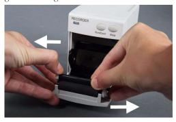
3 Lift up the paper guide on the left side and remove it.
