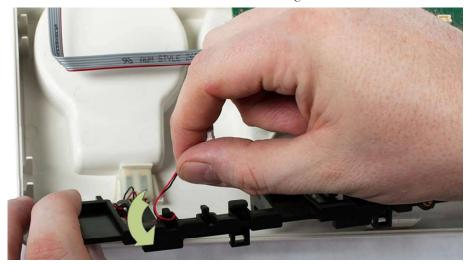
9 Remove the charging contact from its interlock by pressing the springs on each side of it. Assure that the silicon sealing stays attached to the contact.
