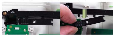
3 With the tool unplug the antenna cable from the antenna board.
