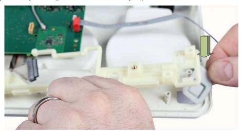
1 Slide the holding frame back in its interlock and fasten the three screws.
