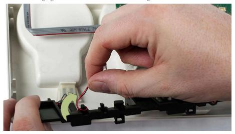
4 Plug the charging connector back into the PCA board.
