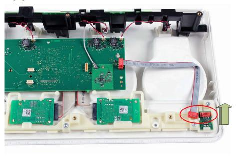
2 Press with the screw driver on the release catch and gently slide the switchboard from its mounting.
