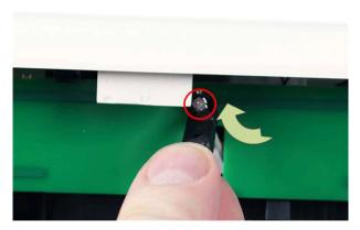
4 Place the antenna removal tool into the designated interlock in the bottom housing with the fork part facing up and bracing against the side wall from the bottom housing.
