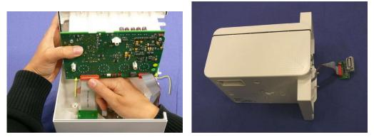
Make sure that the screws in the rear cover are tight enough so that the FMS is properly sealed and that the silicone screw covers in the MMS mount are inserted with the hole facing downwards.
