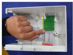
5 Reassemble the MSL UP board by performing the above steps in reverse order. When reassembling, push down MSL holder before tightening screws.
