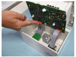
Make sure that the screws in the rear cover of the FMS are tight enough so the FMS is properly sealed.
