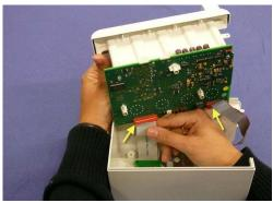
7 Reassemble the FMS by performing the above steps in reverse order. When reassembling the front and back of the FMS, make sure the cables are inserted into the main board as shown below.
