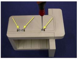
2 Remove the bottom cover. If cable management hooks are installed, remove them.
