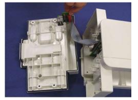
12 Remove the MSL cable from the board.
