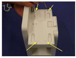
6 Remove the four screws (T10) from the MMS mount.
