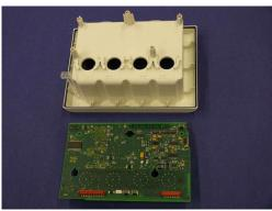
6 Reassemble the FMS by performing the above steps in reverse order. Make sure that the light guide is in its correct position (see picture below) and reinsert the connector holders by pushing them in until you hear a click.
