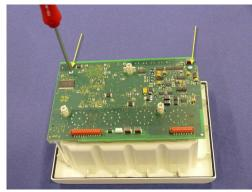
4 Pull out the two connector holders with a flathead screwdriver.
