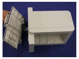
**9** Remove the two screws (T10) from the MSL holder.
