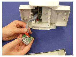
**13** Reassemble the FMS by performing the above steps in reverse order. When reassembling insert the silicone screw covers with the holes pointing towards the bottom.
