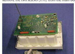
2 Remove the two screws (T10) from the main board.
