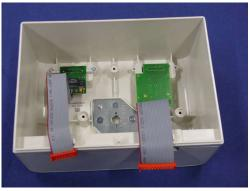
4 Push the MSL UP board forwards to remove it.
