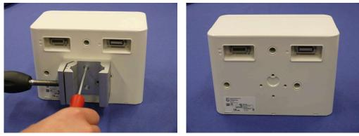
If any other mounting bracket is installed, remove it.
