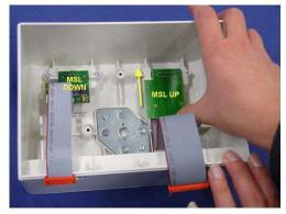
5 Remove the MSL DOWN board accordingly by performing the above steps for the other MSL board.
