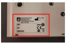
Copy all information onto the new Rear Housing label from the old Rear Housing Label using a waterresistant pen.
