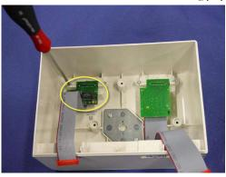
6 Reassemble the MSL boards by performing the above steps in reverse order. When reassembling, push down MSL holder before tightening screws.
