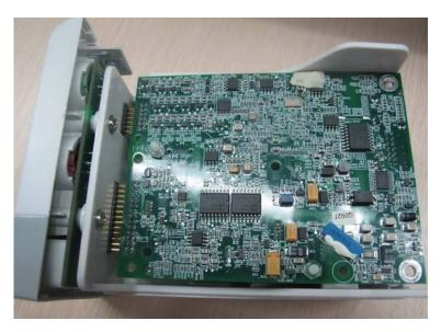
6. Unscrew the two M3×4 screws on the  $SpO_2$  board to separate the  $SpO_2$  board and the parameter board.
