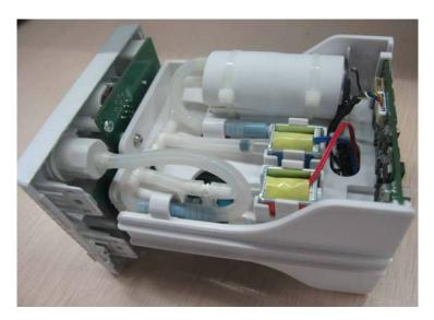
3. Disconnect the cable of the infrared communication board, and release the snap lock to remove the infrared communication board.
