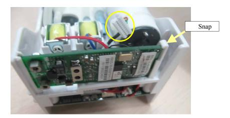
4. Disconnect the cables of the NIBP inflation pump and the relief valves from the parameter board. Snip off the cable ties to remove the pump. Release the snap locks to remove the valves.
