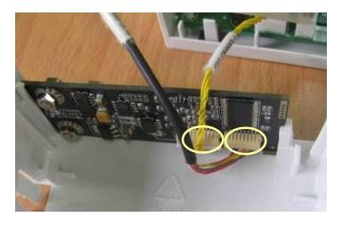
5. Disconnect the cables from the button board and unscrew the PT3×8 screw. Then release the two clips and take out the button board. After that, disconnect the cable to the fan and remove the button board.
