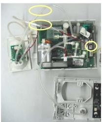
7. Disconnect the tubing between the  $CO_2$  parameter board and the front panel. Then release the four clips and remove the  $CO_2$  parameter board.
