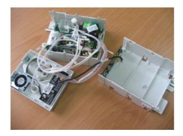
4. Remove the module infrared communication backboard and disconnect all the cables from it.
