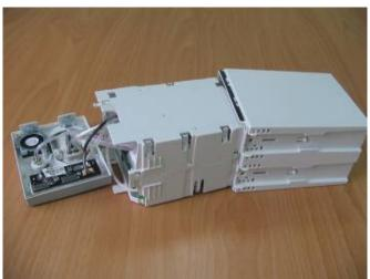
3. Hold the inner housing with both hands. Press the snap side with your thumb and push the other side with the index finger and the middle finger to separate the inner housing into two halves.
