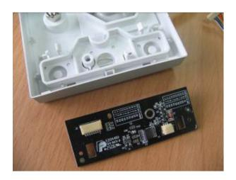
6. Unscrew the two screws on the front panel. Disconnect the tubing between the watertrap assembly and  $CO_2$  parameter board. Disconnect the cable between the watertrap and  $CO_2$  parameter board. Then take out the watertrap connecter assembly.
