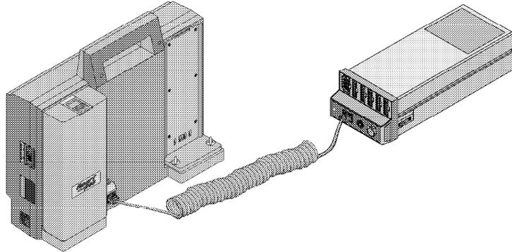
2. Remove the Tram module from the bedside monitor.
