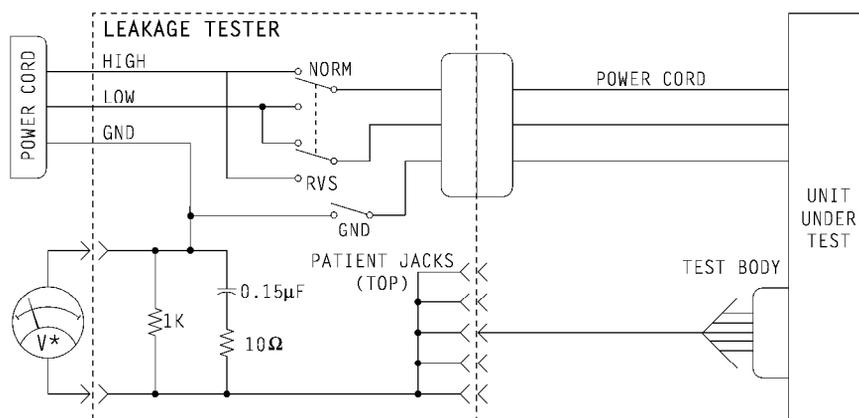
1-mV meter reading = 1-µA leakage current
