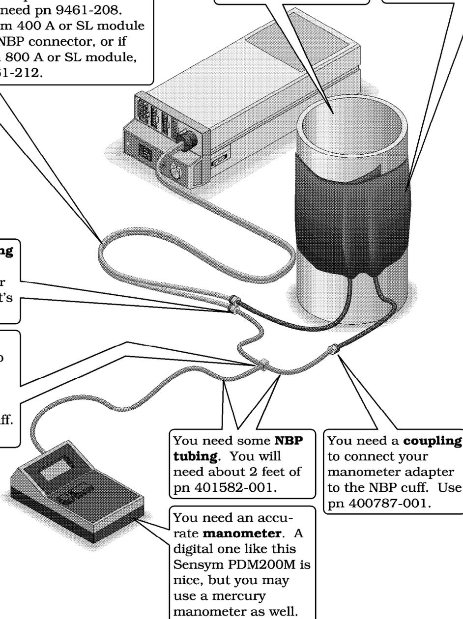
2. Turn the manometer ON, and set its range switch to the 1000 mmHg setting.
