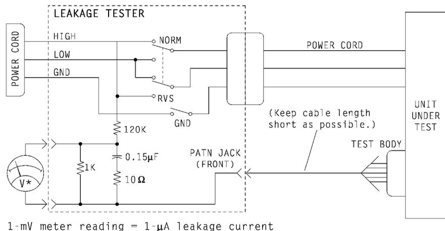
5. Change the leakage tester polarity switch to the RVS position.
