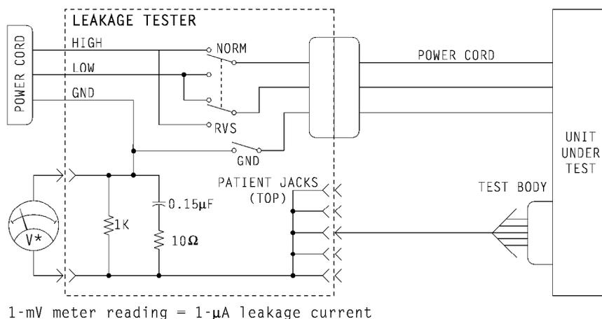
10. Change the leakage tester polarity switch to the RVS position.
