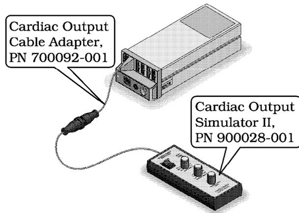
2. Set the cardiac output simulator to output the BT (blood temperature) readings in the following table and observe the correct readings on the monitor:
