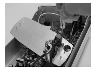
4. Disconnect the UA mode select switch wire from the electronic board. Press on the sides of the UA mode select switch on the back of the front panel and push it outward to remove the switch. Take note of the switch orientation in terms of its wires colors to prevent incorrect switch orientation at the time of re-installation.
