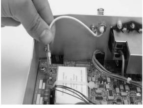
6. Use a small wrench to remove the nut that fixes the antenna connector to the rear panel to remove the connector.
