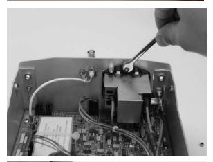
5. Disconnect the antenna wire connector from the main board by firmly holding the connector end of the wire and pulling it upward.
