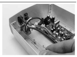
4. Disconnect the power connector going to the power supply board to remove the power module assembly.
