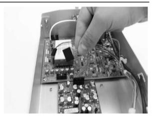
4. Disconnect the antenna wire connector from the main board by firmly holding the connector end of the wire and pulling it upward.
