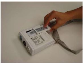
3. Move the battery out and disconnect the battery wire from the Mini Telemetry electronic board to remove the battery.
