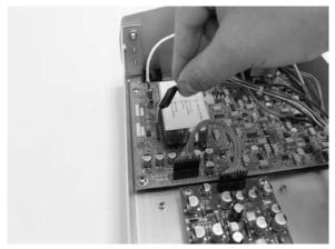
3. Disconnect the power header connector from J1102 connector on the main board.
