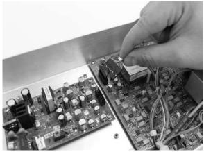
4. Use a Phillips screw driver to remove the four screws attaching the power supply board to the chassis and then remove the board.
