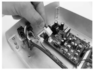
3. Disconnect the output power header connector from P2 connector on the power supply board.
