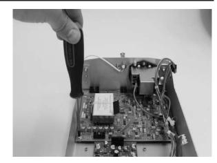
8. Cut the tie wrap attaching the radio module to the main board and pull out the radio module to disconnect it from the main board.
