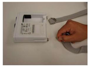
3. Use a T10 Torx screw driver to remove the two screws on the side of the transmitter case and remove the bottom cover.
