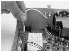
5. Disconnect the UA switch / LED wire connector from from the main board.
