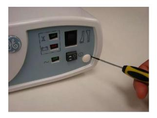
2. Use a T15 Torx screwdriver to remove the two screws on the front panel and the two screw on the sides of the top cover.
