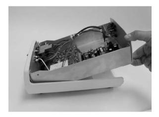
2. Use a small nutdriver to remove the 3 nuts fixing the rear panel to the chassis.
