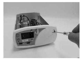
6. Use a T15 torx screw driver to remove the two screw on the rear panel.
