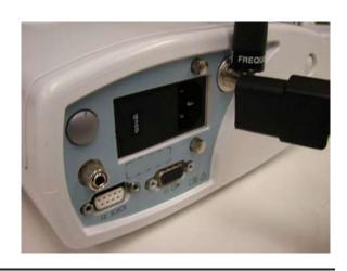
2. Use a small screw driver to open the fuse holder compartment of the power module on the rear panel of the receiver.
