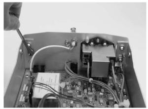
3. Use a 5mm nut driver to remove the hex screws attaching the D9 connectors (J1, J2) to the rear panel.
