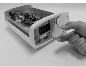
5. Use a small screw driver to remove the screw caps on the bottom cover at the rear side of the unit.
