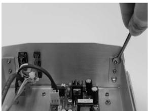
3. Use a small Phillips screw driver to remove the two screws attaching the power switch to the panel to release the power switch.
