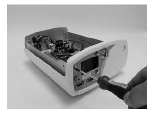
7. Use a 3mm hex key to remove the four screws on the bottom side of the receiver.
