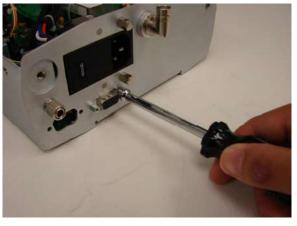
7. Use a Phillips screw driver to remove the four screws attaching the main board to the chassis and then remove the board.
