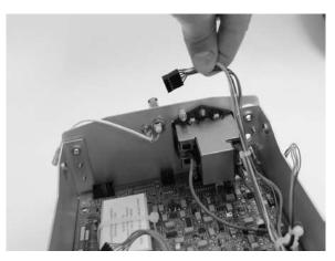
6. Use a 5mm nut driver to remove the hex screws attaching the D9 connector J1 to the rear panel.
