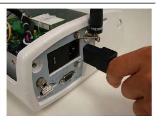
3. Disengage the receiver antenna from antenna connector and put it aside.
