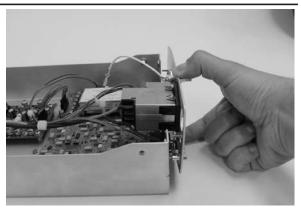
2. Use a wire cutter to cut the power cable tie and release the power cable.
