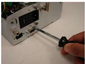
4. Use a small wrench or nut driver to remove the 4 screws attaching the power module to the rear panel to release the power module. Use a nut driver to remove the nut attaching the equipotential lug to panel to release the lug.
