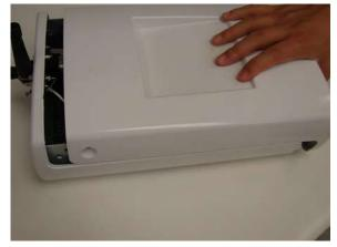
2. Use a small wrench or nut driver to remove the 4 nuts fixing the front panel to the chassis.
