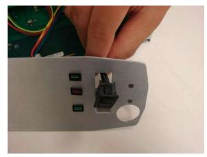
5. Use a small screwdriver to press on the sides of the grommet collars on the back side of the panel and pull the grommets out to release the LED's.
