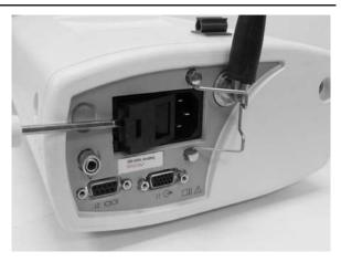
3. Use a small screwdriver to slide the fuse holder out and replace the fuses.
