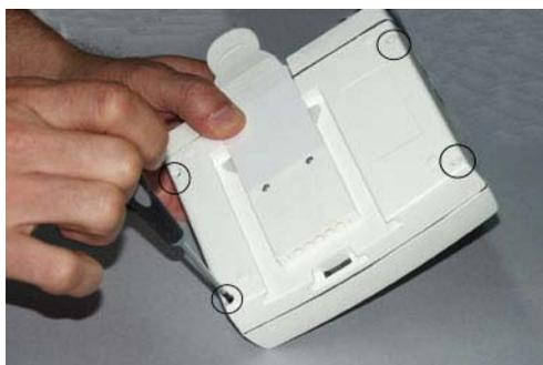
1. Remove the four screws (T8) holding the module cover to the frame from the bottom of the module.
