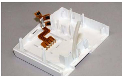
21. Pull the module bus connector carefully through the hole in the frame.
