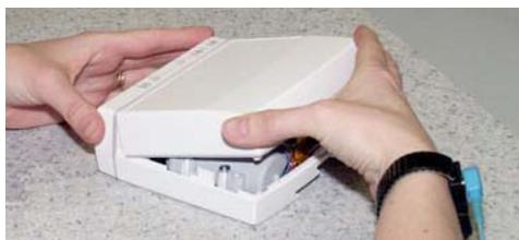
2. Hold the cover from the back corners, lift it about 45° to unlock the snaps from the front unit and pull the cover out backwards.
