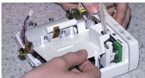
8. Remove the STP-ECG insulator plate. Be careful not to damage the NIBP hoses.
