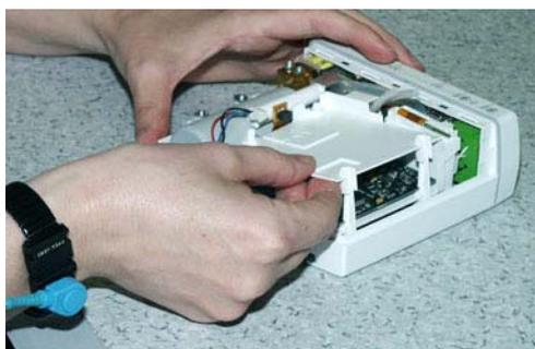
5. Lift the NIBP-STP insulator plate carefully up.
