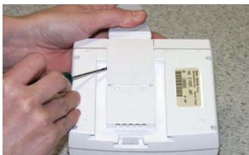
13. Flip the module over and remove the two (T6) screws holding the lock unit to the frame. While pulling the tab push the lockers with a screwdriver to remove the lock unit.
