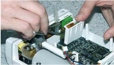
9. Hold down the ECG board for example by pressing the ECG input unit and use pincers to disconnect the ECG input flex connector from the ECG board.
