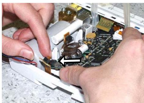
7. Lift the STP board a little to disconnect the module bus connector. Remove the STP board.
