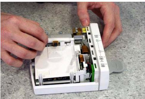
2. Remove the NIBP filter cover and replace the filter.
