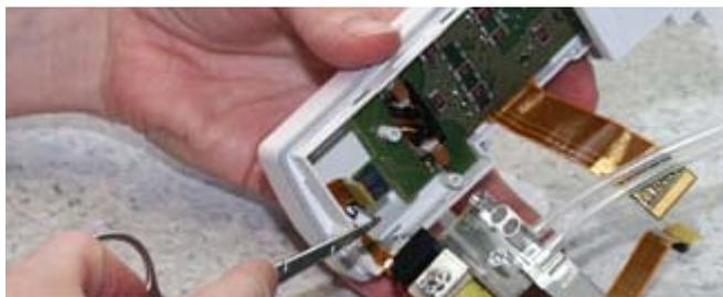
19. Lift the manifold carefully aside. Be careful not to damage the NIBP flex board. Disconnect the NIBP flex board connector from the STP input board.
