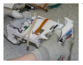
Detach the front chassis unit from the module frame. Be carefull not to damage the NIBP flex board.
