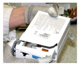
2. While pressing the release latch, pull the module cover slowly backwards and remove it from the main body.
