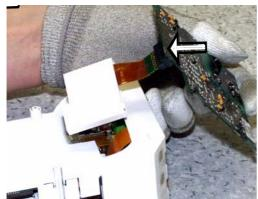
Disconnect the ECG input flex connector from the ECG board. Be carefull not to damage the flex.
