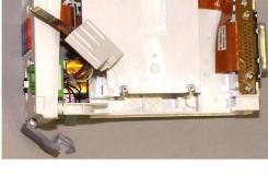
Disconnect the module bus connector from the STP board.
