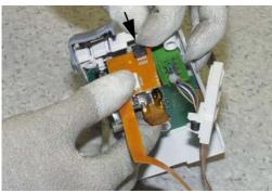
Disconnect the NIBP flex board connector from the STP input board. Lift the manifold carefully aside. Be careful not to damage the NIBP flex board.
