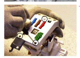
Remove the three screws (T8) holding the front chassis to the module frame.
