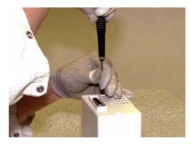
1. Remove the two screws (T8) holding the module cover to the module frame from the back of the module.
