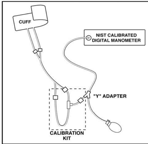
**Leak Test Setup**
