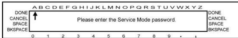
6. A row of numbers is displayed at the bottom of the screen. Turn the Trim Knob and move the arrow to the desired number, then press the Trim Knob to select the number. Enter the Service Mode password, **2213**.
