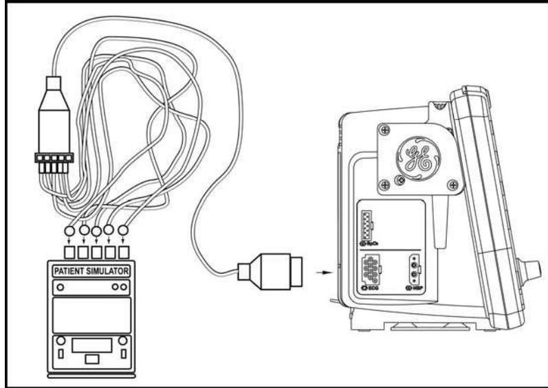
1. Set the ECG simulator to output a Paced ECG Waveform.
