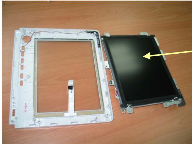
2. Unscrew the four M3×6 screws underneath the screen cover and then remove the LCD.
