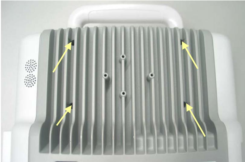
2. Unscrew the three M3×12 screws and remove the power supply cover.
