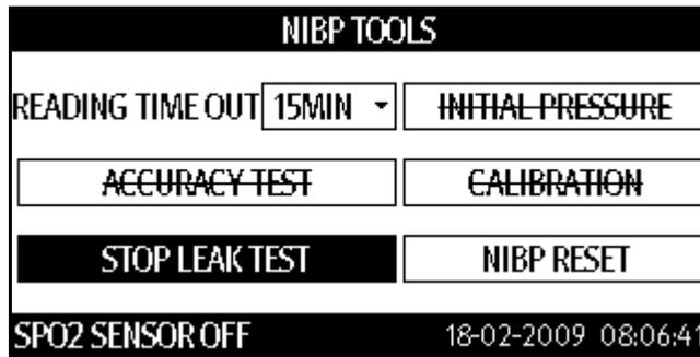
**FIGURE 6-12** NIBP TOOLS dialog running the leak test
