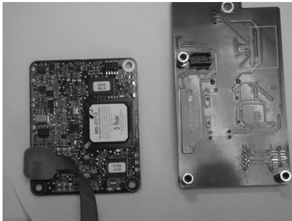
FIGURE 4-31 Masimo SpO 2 board and isolated power supply.
