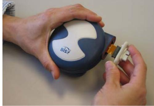
1. Disconnect BISx from the monitor and remove Patient Interface Cable from BISx.
