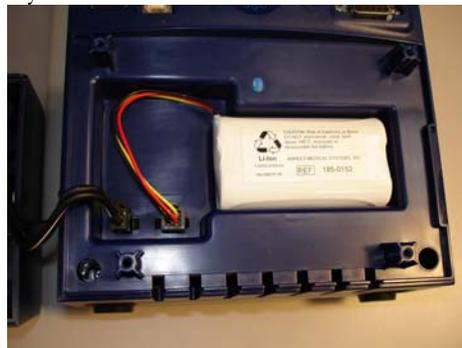
5. Lay the new battery in the recess with the wires at the top, and plug in the connector.
