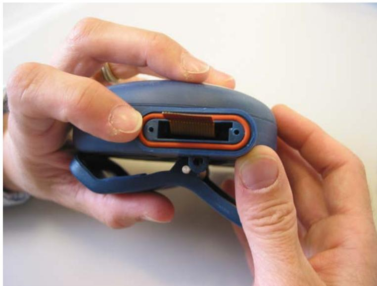
5. Set the new gasket in the groove of the BISx housing.
