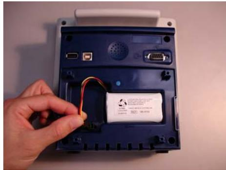
3. Remove 4 screws from the Battery/Power Supply cover and remove the cover. Note the position of the battery cable.
