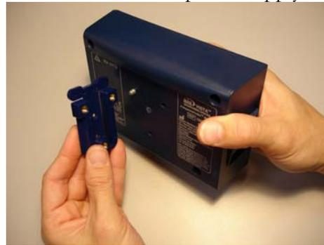
6. Remove the three screws that attach the Clamp Shoe to the back panel.
