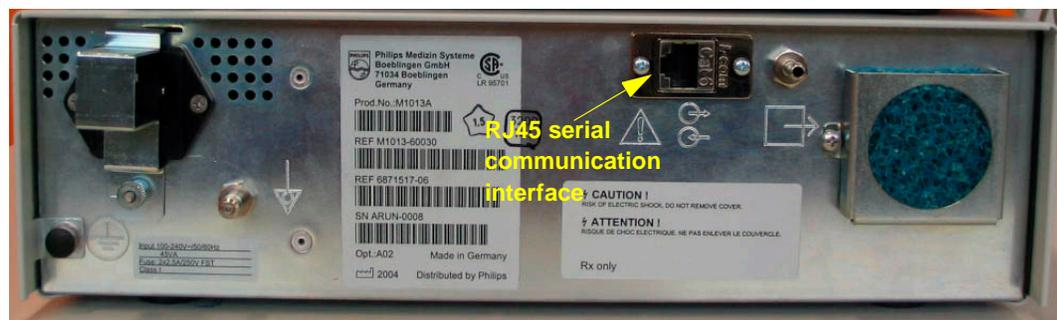
Figure 4 RJ45 connection on the back of the gas analyzer
