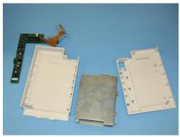
7 To reassemble the battery extension, perform the above steps in reverse order. Always make sure that you do not damage the flex cable.
