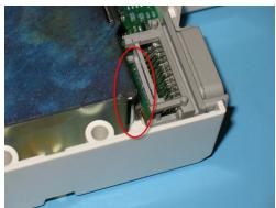
6 To remove the main board, lift it up as shown below and then pull it out. When replacing the main board, make sure that the small LED board (circled in red below) is positioned correctly.
