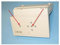
2 Lift up the front cover of the rear housing as shown below and slide it out. Be careful not to damage the flex cable.
