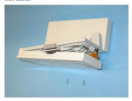
The front cover of the rear housing and the metal plate are now accessible.
