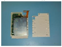
Now the battery cage can be lifted out of the housing.
