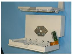
3 Unscrew the two screws on the bottom of the housing using a Torx T10 screwdriver.
