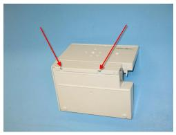
The back part of the rear housing is now accessible. If you need to replace this part, make sure you transfer the serial number tag to the new housing part. Be sure not to lose the pins holding the housing together, as you will need them for reassembly.
