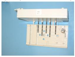
4 To disassemble the bottom housing, open the battery door and pull out the plastic pin as shown below.
