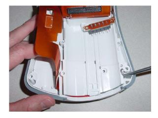
4. Remove the ePort connector attached to the flex circuit assembly from the bottom housing.
