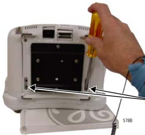
Note: Use a screwdriver with a long blade or remove the GCX plate first for easy access to the bottom screws.
