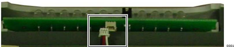
6. Carefully remove the defective alarm light PCB and set aside.
