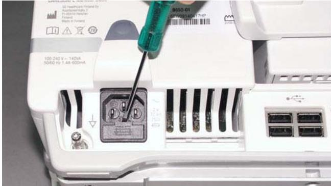
The mains fuses are situated on the back of the monitor, below the mains connector.
