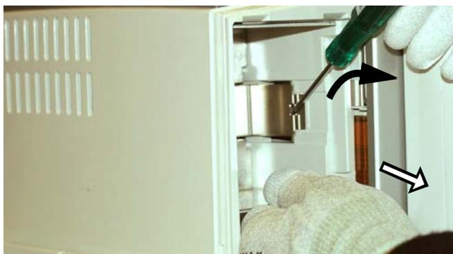
5. Release the snaps in the recorder EMC cover with a flat blade screwdriver while simultaneously pulling the bottom plate of the EMC cover.
