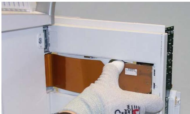
3. Disconnect the Hinge Flex Board from the Module Frame connectors.
