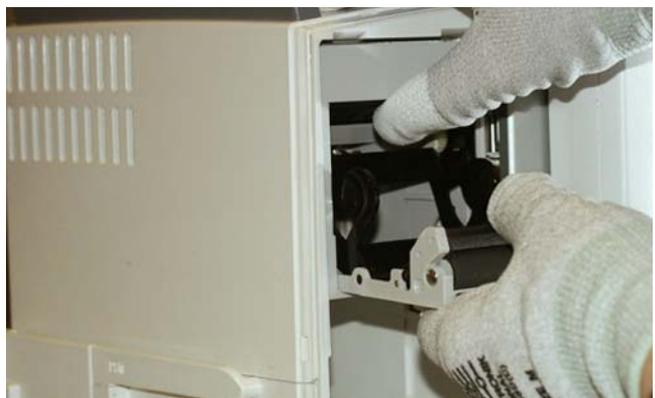
4. Pull the recorder carefully out of the Module Frame.
