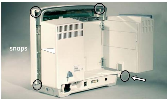
3. Remove the four T10 screws in the top and bottom corners behind the Display Unit. [Torque 0.6 Nm]
