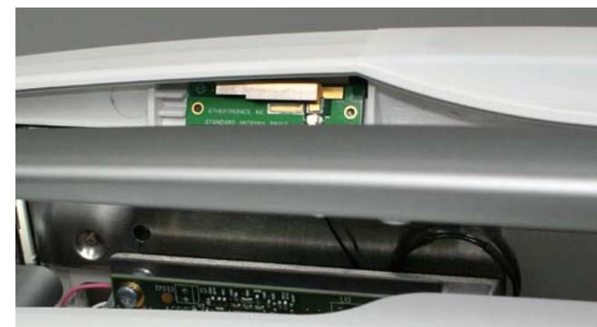
4. Make sure the contact area for the antenna board adhesive in the Front Unit Assembly is clean and free of grease.
