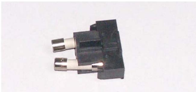
2. Pull the fuses out of the fuse holder and insert new ones.
