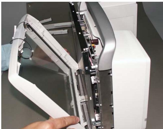
7. Disconnect the U/I cable from the User Interface Board.
