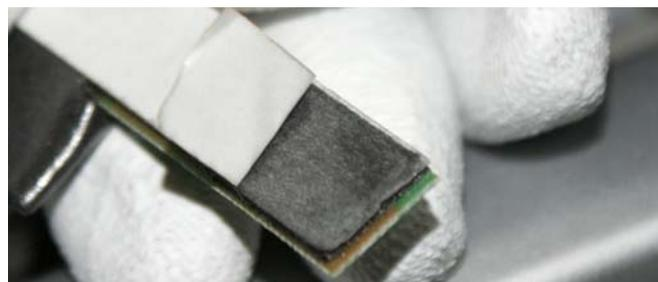
3. Peel off the paper release liner from the antenna board mounting tape one at a time (see steps 3 and 4 below).
