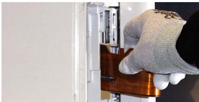
6. Detach the Module Frame back plate and disconnect the Hinge Flex Board from the Module Frame connectors, see section [12.2.5](#).
