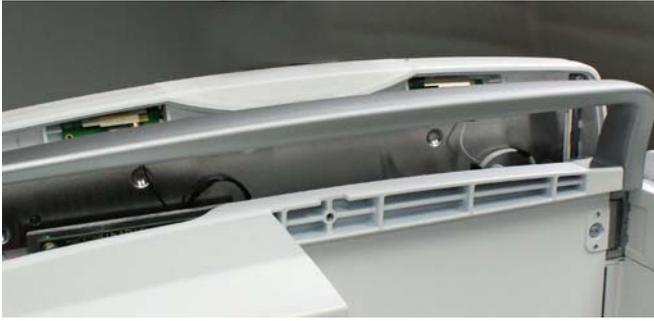
NOTE: Place the antenna cables carefully as shown in the pictures.
