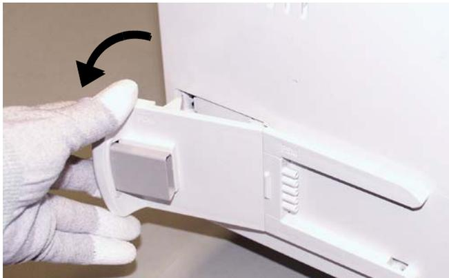
3. Turn the PDM Docking Mechanism to a 30° angle to detach it from the Module frame flex board connector.
