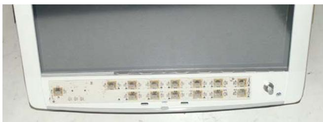
3. Tear the membrane keypad from the Front Unit and detach the keypad connector that connects it to the User Interface Board.
