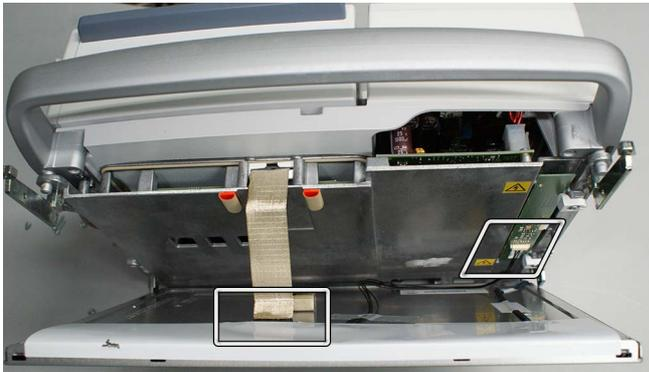
3. Detach the LVDS cable from the LCD display.
