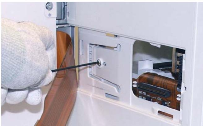
1. Detach the Module Frame back plate and the Hinge Flex Board from the Module Frame connectors
