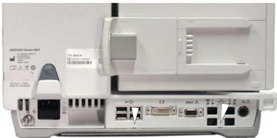
1. Detach the Interface Board cover plate from the frame by releasing the snaps with a flat blade screwdriver.
