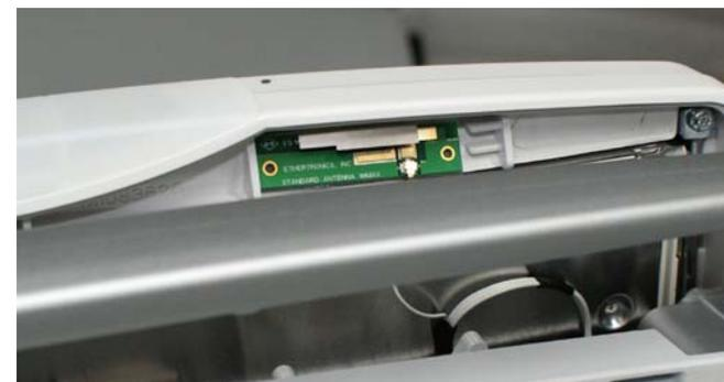
5. Make sure the contact area for the antenna board adhesive in the Front Unit Assembly is clean and free of grease.
