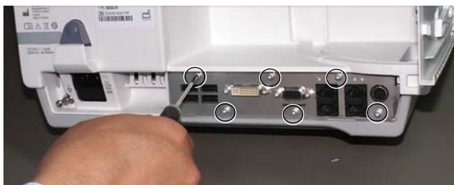
2. Remove the six T10 screws that hold the Interface Board to the main unit.
