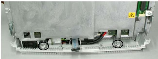
5. Remove the two T10 screws with washer insulators mounting the Base Unit to the mid-frame. [Torque 0.8 Nm]
