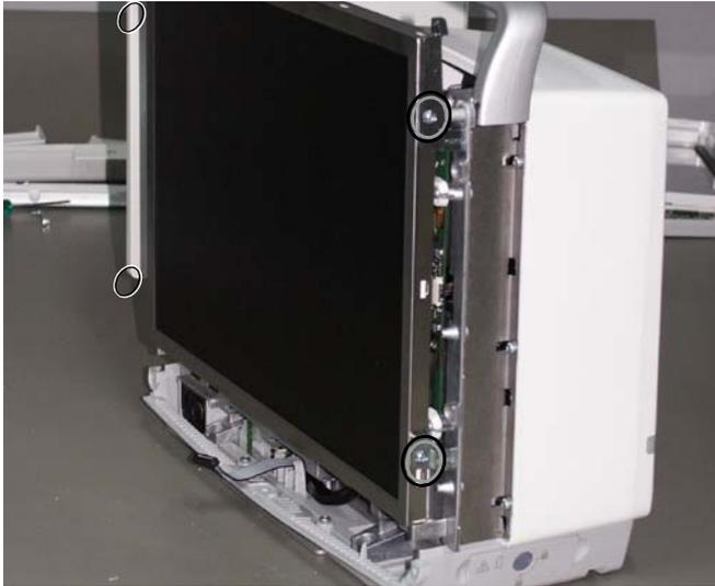
1. Detach first the Front Unit Assembly, see section [12.4.1](#).
