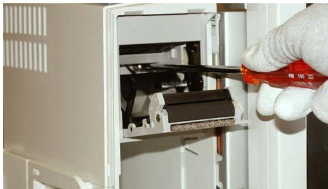
1. Detach the Module Frame front cover, see section [12.2.1](#).
