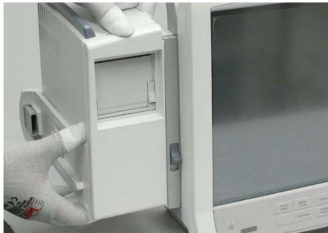
3. Press with finger from the top of the PDM docking rail.
