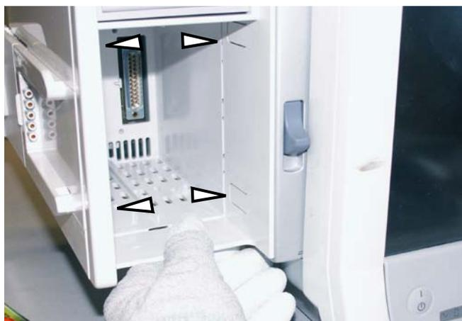
3. Release the four snaps in the inner side of the E-module slot by pressing them (inwards) with your finger. Release first the topmost two snaps and then the lowest two snaps.
