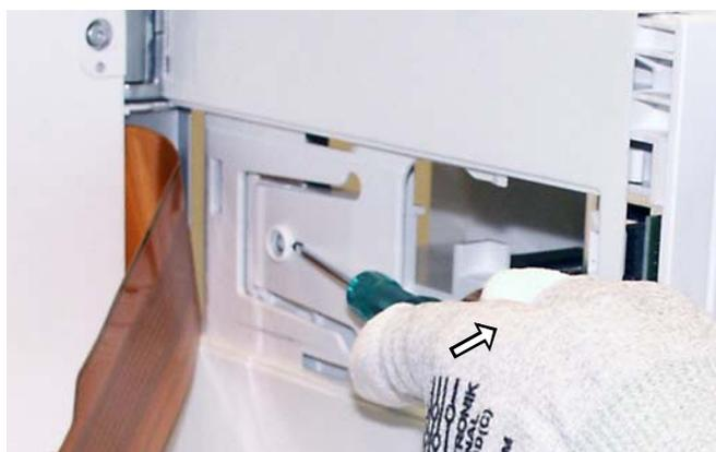
3. Release the snap behind the flex cable. Lift the flap with a flat blade screwdriver.
