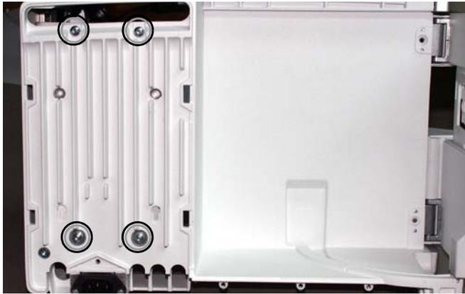
7. Remove the four T10 screws mounting the AC/DC board to the back plate.
