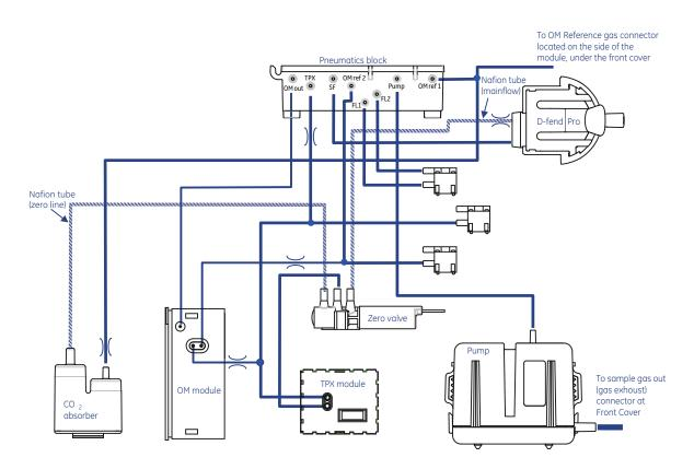
NOTE: The nafion tubes do not include the silicon fittings they connect to. Use the original silicon fittings unless they are damaged or leaking.
